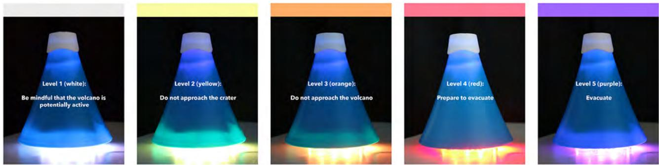
Figure 4: The first prototype of our Fuji-chan device. The model is 12cm high and 11cm in diameter at the base. The light at the top indicates the weather conditions (in this case, each image shows white: between  $-10$  and  $0^{\circ}\text{C}$ ) at the summit of the mountain, while the lights at the bottom indicate the volcanic eruption risk level (levels 1-5 are shown). Aural feedback via a piezo speaker inside the model is also provided for levels 2 and above.
