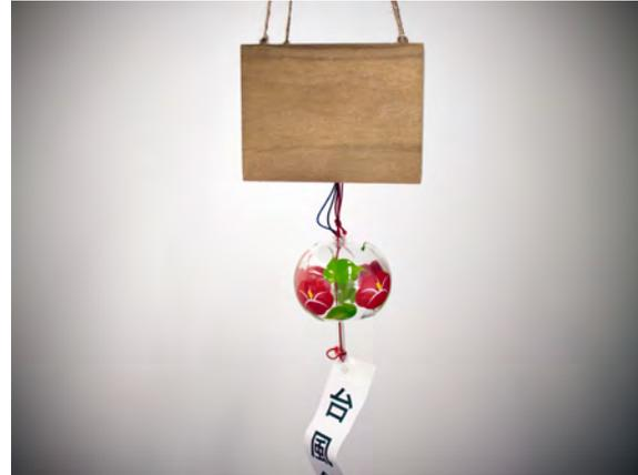
**Figure 3:** The exterior of our Taifūrin system. The box contains a Raspberry Pi [12], its power source, a servo motor and an LED (See Figure 4). Below the box hangs a traditional Japanese wind-chime (fūrin), which is attached to the servo motor and the LED, which is placed inside the bell. By relying on natural materials and creating a simple interface, we consider this design artefact to incorporate wabi-sabi aesthetics.
